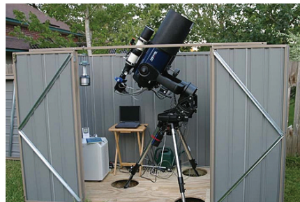
Russ's earlier backyard observatory, first with a Meade 10" and later fitted with a 14 inch RC, both using an ST-10XME
